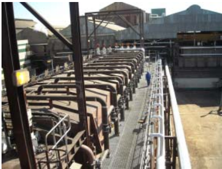
Lateral view with juice distributors feeding pipes
